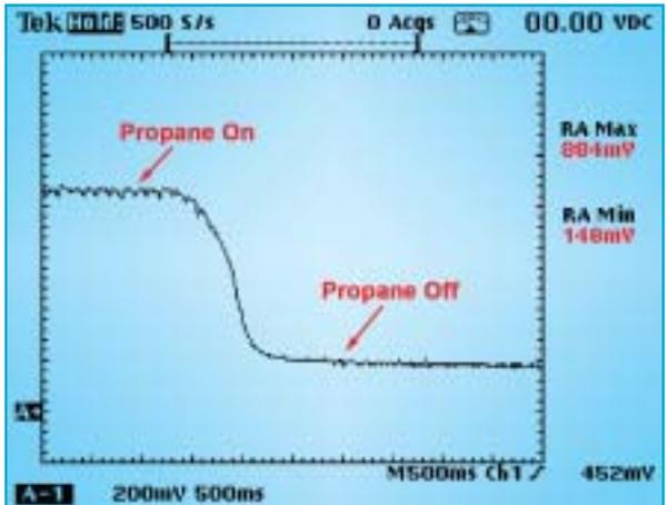
Figure 10 — Here's the signal you're looking for using a propane enrichment tool to force the system rich.
