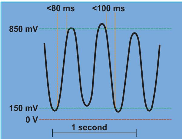
Figure 5 — Here's what you're looking for in a good oxygen sensor: Voltage limits, rise and fall times. And the voltage should never drop below zero.
