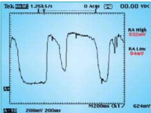
Figure 8 — If the fuel system is in good condition and working properly, you can verify the oxygen sensor simply by goosing the throttle a few times.
