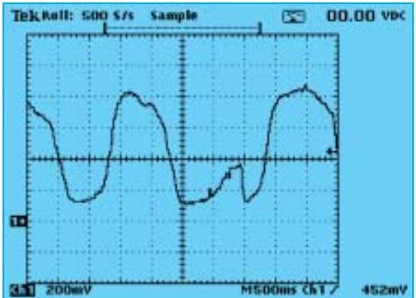
Figure 6b — The same oxygen sensor as before, but this time the scope was connected to the sensor ground instead of the system ground.
