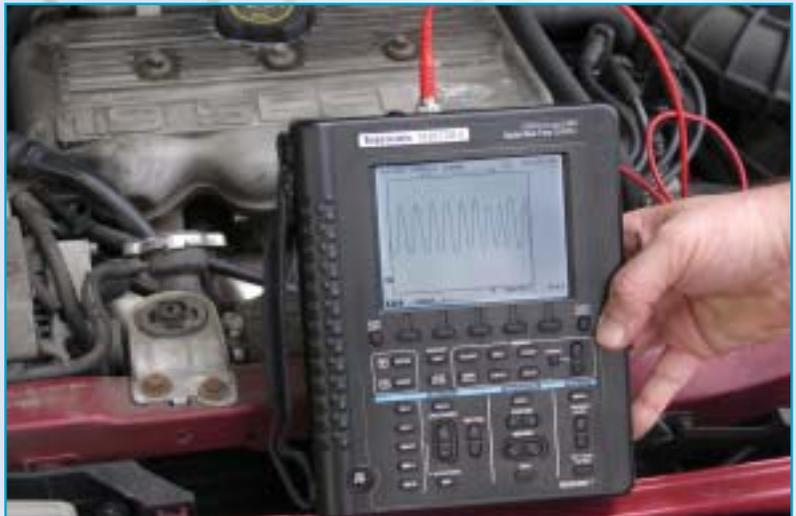
Figure 1 — No other tool provides more information about an oxygen sensor's condition than a digital oscilloscope.
