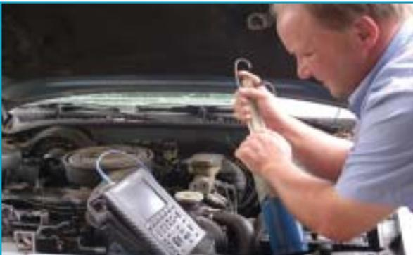
Figure 9 — If you can't get the system rich enough by goosing the throttle, a propane enrichment tool is the easiest way to force the system rich.
