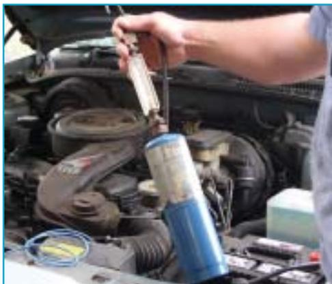
Figure 3 — If the fuel system isn't providing adequate response to the throttle, you may need a propane enrichment tool to force the oxygen sensor rich.
