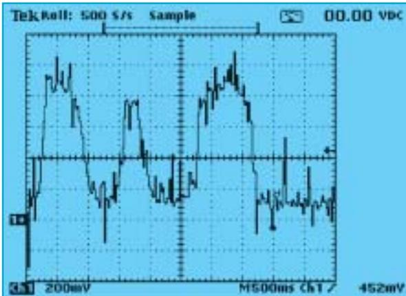
Figure 6a — Here's the signal you might see if you've connected your scope to the system ground instead of the oxygen sensor ground.
