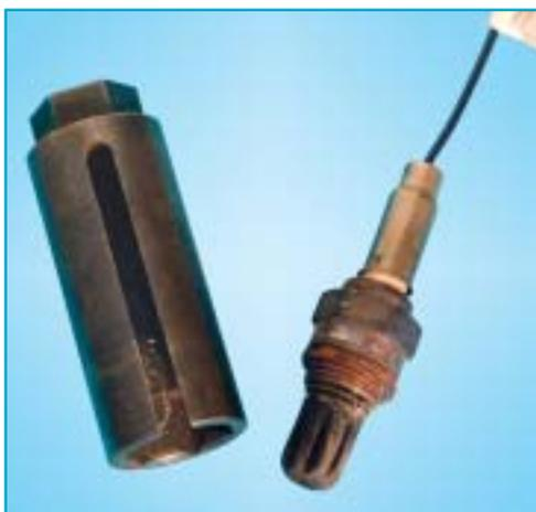
Figure 4 — Not a necessity, but nice to have around, an oxygen sensor socket makes removing the oxygen sensor easier.
