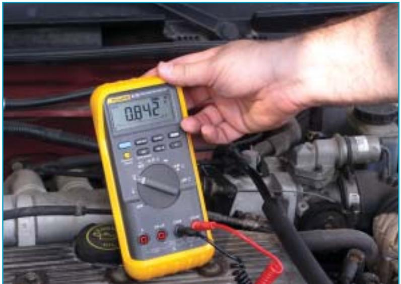
Figure 2 — You can use a digital meter to check the oxygen sensor's condition, but you won't be able to measure rise and fall times.
