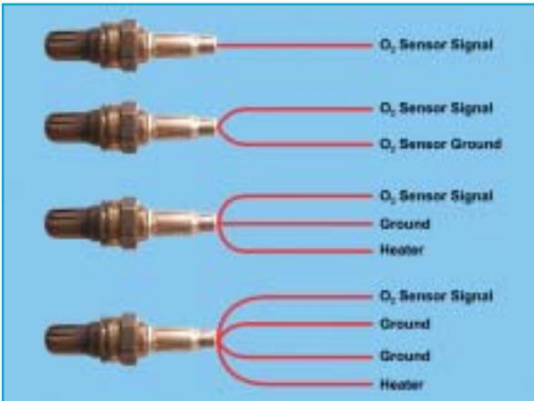
Figure 7 — Most of the time, finding the sensor ground is easy. The only problem is on a 4-wire sensor; for that, take your ground from another sensor altogether.
